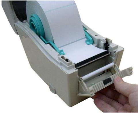
1. Refer to section 3.2 to load the media. Open the top cover and peel-off panel after calibrating the sensor.
