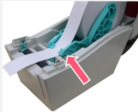
5. Place the paper, printing side face up, through the media guides, media sensor and place the label leading edge onto the platen roller.
