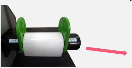
4. Place media roll on label supply spindle. Replace label roll guard. Make sure the label roll guard position of each sides are the same as the length of the label. Please check the outside edge scales are both close to the label width.
