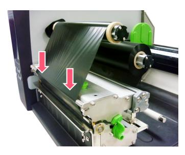
6. Close the print head mechanism making sure the latches are engaged securely.
