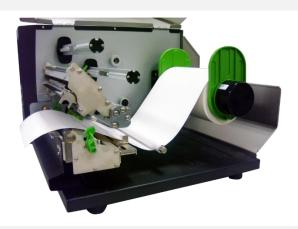
**5.** Pull label roll leading edge forward through the media guide bar, media sensor (green) and place the label leading edge onto the platen roller.
