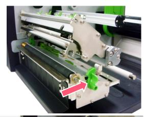
**1.** Lift the handle to open the printer right side cover. Push the print head release lever to open the print head mechanism. Please refer to section 3.3 to load media.
