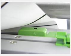
6. The media sensor position is moveable. Please make sure the gap or black mark is at the location where media gap/black mark will pass through for sensing. Note:
