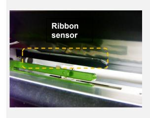
Thread the ribbon through the ribbon sensor slot and then through the open space in between print head and platen roller.
