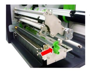
Lift the handle to open the printer right side cover.
