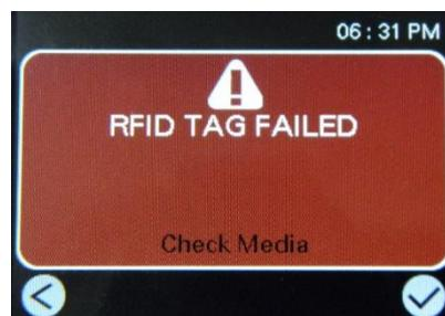
If you need to overwrite this locked tag, please use RFID READ unlock command as following programming example, to unlock password for the RFID tag so it can be overwritten later.
