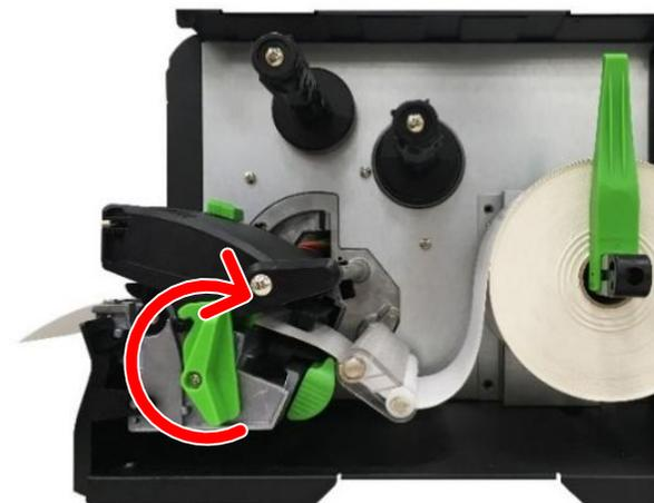
5. Adjust the media sensor location ensuring that the sensor can detect the media.
