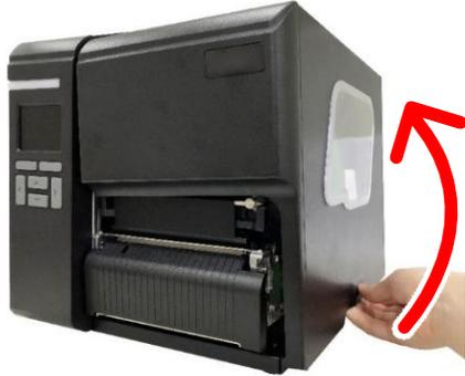
2. Load the ribbon and media roll. For how to load the ribbon and media roll, please refer to [Loading the Ribbon](#) and [Loading the Media](#).
