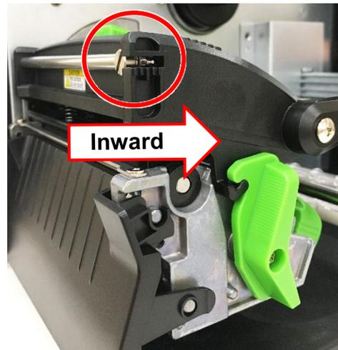
1. Switch the ribbon tension adjustment knob clockwise per 1 level and print the label again to check if the wrinkle is gone.
