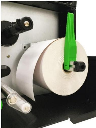
4. Rotate the lever as indicated to release the printhead and then thread the media underneath the damper, through the media sensor, and label guide.
