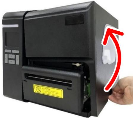
2. Load the ribbon and media roll. For how to load the ribbon and media roll, please refer to [Loading the Ribbon](#) and [Loading the Media](#).
