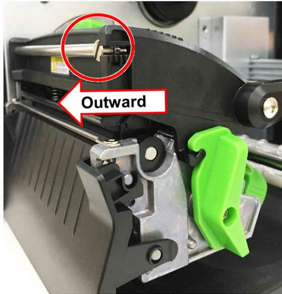
1. Switch the ribbon tension adjustment knob counterclockwise per 1 level and print the label again to check if the wrinkle is gone.
