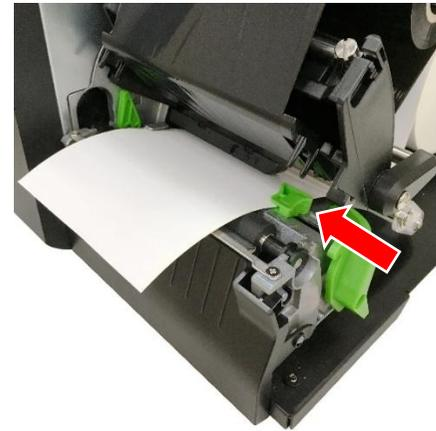
7. Press down to close the printhead mechanism ensuring that the printhead mechanism is correctly secured in place.
