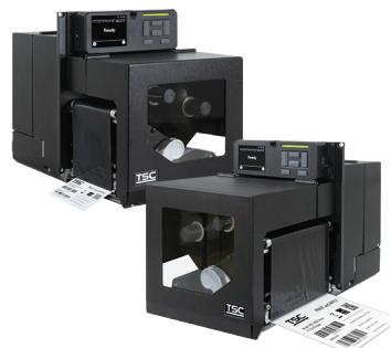
The PEX-2000 Print Engine seamlessly combines high-performance RFID encoding with exceptional reliability in a compact design for automating item-level RFID tagging. With a rich legacy, it effortlessly incorporates into any print and apply system, providing a comprehensive solution.
