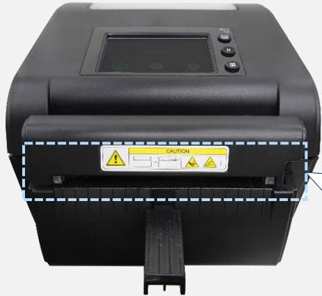
The cutter blade has sunk into the chassis after turning on the printer.
