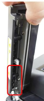
Please ensure that any residue in the crevice of the cutter upper bar is also removed with the sponge foam swab.
