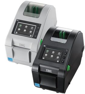
The DH220L RFID is an HF/NFC RFID printer for applications requiring short-range secure scanning, handling 10-60 mm wide labels on rolls up to 6.5-inch OD. Available in standard and medical-grade antibacterial versions, it's ideal for wristbands, blood bags, and other long, narrow labels.
