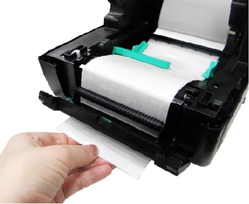
A side view of the printer with the lid open. The white backing is now inserted into the slot in the lid. A hand is shown holding the end of the backing. |
