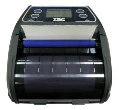
Press each side of media cover to close the media cover and make sure the media cover closed correctly.
