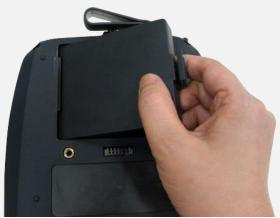
**2.** Insert the left side to install the battery at the rear of the printer.
