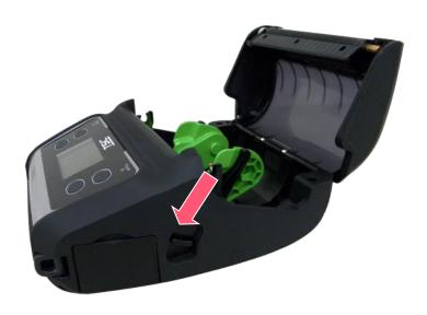
**1.** Open the printer media cover by pressing the media cover release button.
