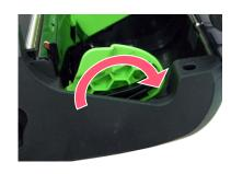
2. Push down each side of media holder lock switch to fix the media holder..
