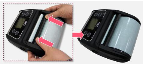
**6.** Move the peeler module to near the peeler bar by pushing each side of peeler module. (cover the platen roller)
