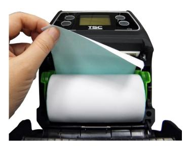
3. Place the roll between the media holders and close them onto the core. Place the paper, printing side face up, and pull out enough paper over the print head.
