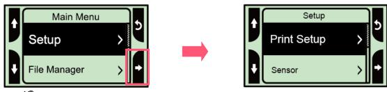
2. Press 🗓 button to enter the "Print Setup" item. Select the "TSPL2" item. Enter the "Speed" setting mode.
