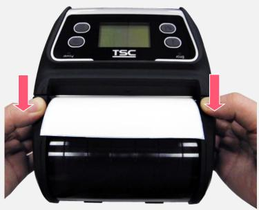
Press each side of media cover to close the media cover and make sure the media cover closed correctly.
