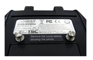
1. Tighten 2 screws on the printer.
