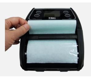
**4.** Feed the liner go through the peeler module. (as figure shown)
