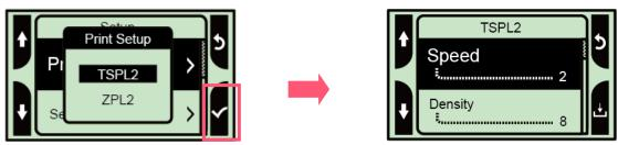
**3.** At this status, you can scroll up or scroll down to select the value of print speed. Then press the button to save the selected value into the printer. Press "butter to back to "Ready mode".
