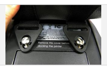
**2.** Put the nut on the media holder. Pull up the belt strap to lock it on the screws.
