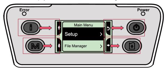
You can use this 4 buttons to scroll, select, enter or return the menu, depend on the icons from 4-sides of LCD. It was selected if the item with the black ground on the screen. The icon function is listed as below,
