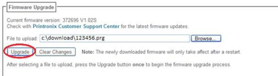
Figure 2 Uploading Firmware File for Upgrade
