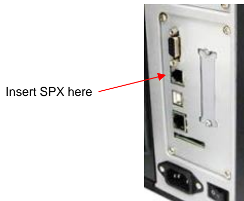
Figure 15 Inserting The SPX into the Debug Port
