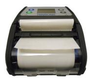
Route the liner under the label peel cover as shown
