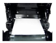
Route the media, printing side out, through the bottom external label slot
