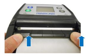
Push the label peel cover toward the front of the printer until it covers the plate roller
