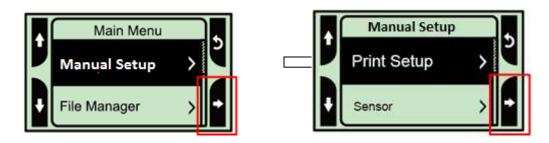
Press the Feed key to enter the "Print Setup" item. Press the Feed key to select the "General" item and display the "Speed" setting mode.
