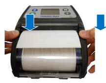
Press down on both sides of the media cover to ensure it is closed correctly.
