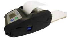
Press down on both sides of the media cover to make sure it is closed correctly
