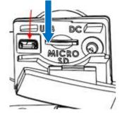
Open the interface cover and connect the printer to the computer/smart phone (host terminal) with USB cable (USB to USB or USB to RS-232).
