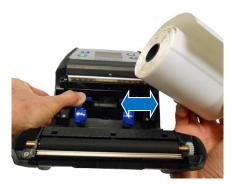
Pull the media holders apart far enough to fit the width of the label roll you are installing
