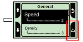
Press the Feed key 1 to enter to highlight the current speed setting. At this status, you can scroll up or scroll down to select the value of print speed. Then press the Feed key 1 to save the selected value into the printer. Press the Power key 1 multiple times to go back to "Ready mode".
