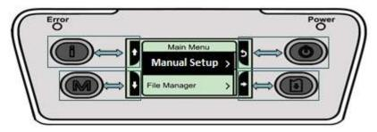
Use the 4 keys at the sides of the LCD to scroll, select, enter or return from the menu. The icon functions are listed below.
