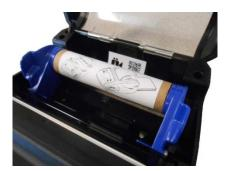
Install Media Core that is the width of your media to secure the media holders in place
