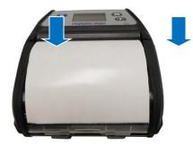
Press down on both sides of the media cover to ensure it is closed correctly.
