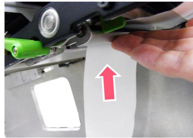
**6. Close print head release lever and label guide bar release lever and press Feed button to test.**
