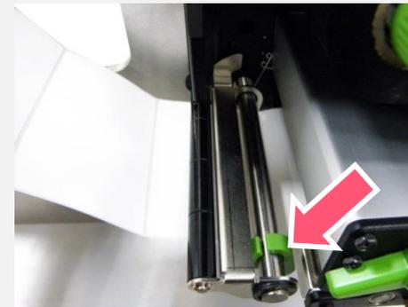
**5. Adjust the front label guide (green) to fit the label width.**
