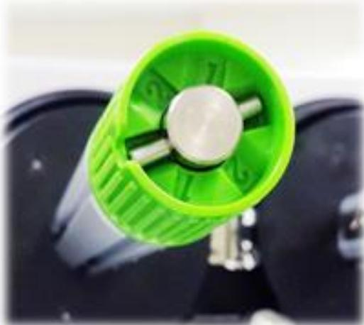
**Ribbon Supply Spindle Tension # 3**
