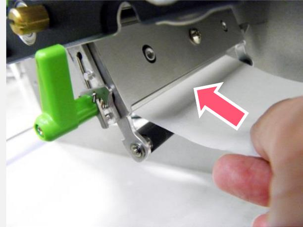
**5. Press the roller to close the peel-off roller release lever.**
