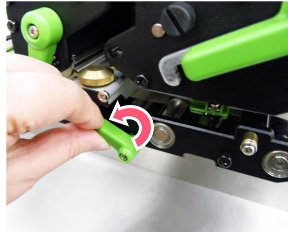
**4. Feed the leading edge of liner through the peel-off roller.**
