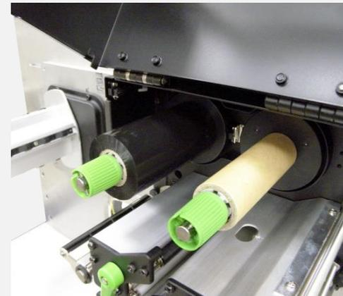
**3. Install the ribbon and paper core onto ribbon supply spindle and ribbon rewind spindle.**
