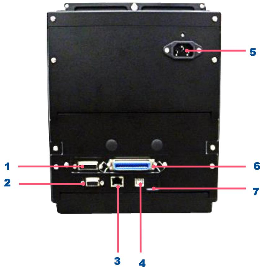
1. GPIO interface (Applicator interface with DB15F connector +5V I/O)
