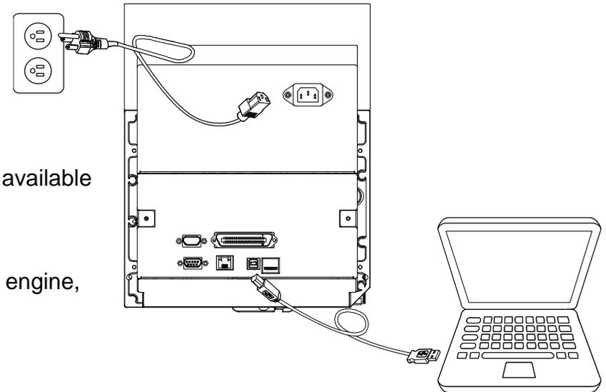
◆ **Note: Please switch OFF the printer before plugging in the power cord to printer power jack.**
