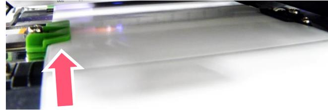
**6. Move the media sensor by adjusting the media sensor position adjustment knob, make sure the sensor is able to sense the media.**
