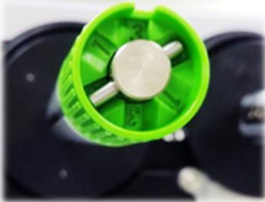
**Ribbon Supply Spindle Tension # 2**
