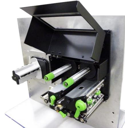
2. Install the ribbon and paper core onto ribbon supply spindle and ribbon rewind spindle.
