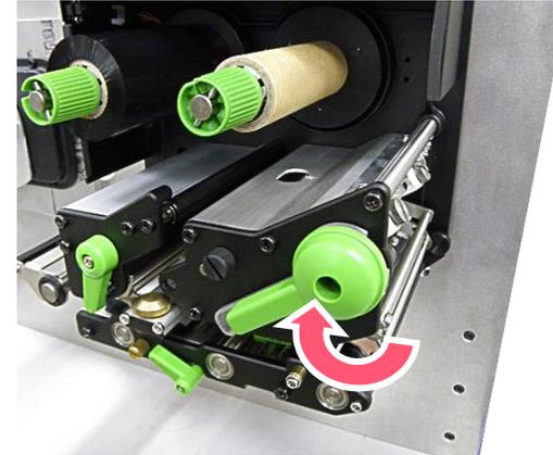
**4. Thread ribbon above the ribbon guide bar and through ribbon sensor slot.**
