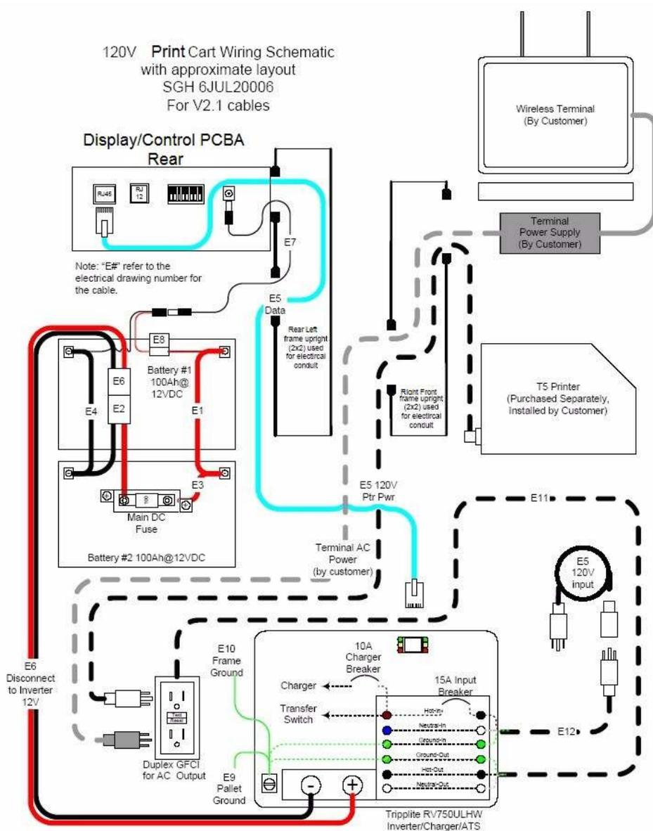
Figure 26. Wiring Schematic for North American Models (120V/60Hz)
