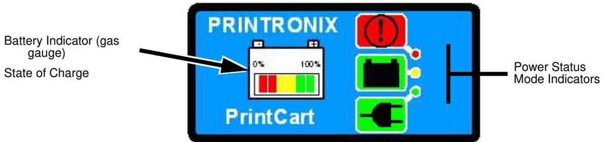
**Figure 10. Display Panel Layout Indicator Colors**
