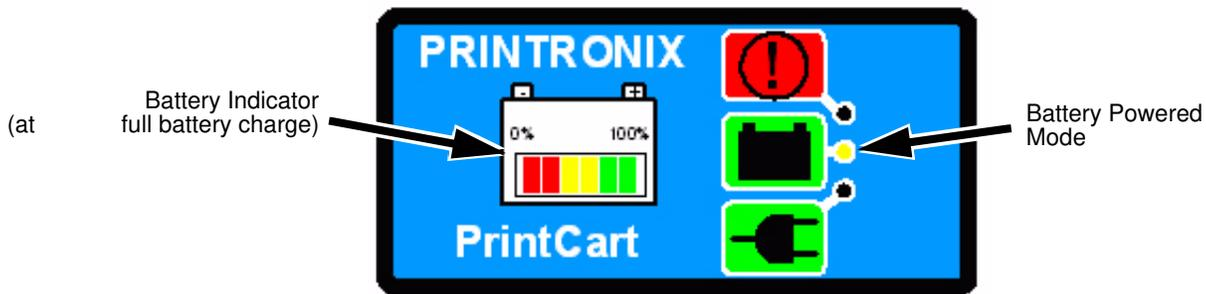
**Figure 11. Operating in Battery Powered Mode with a Full Battery Charge**
