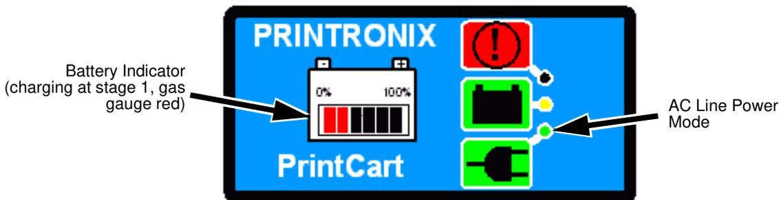
**Figure 12. Operating in Unrestricted, AC Line Power Mode**
