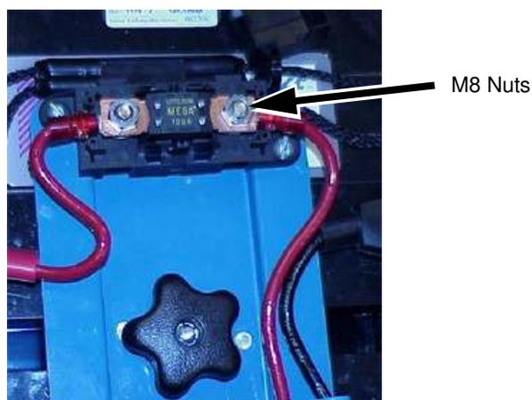
Figure 23. Replacing the Main DC Power Fuse
