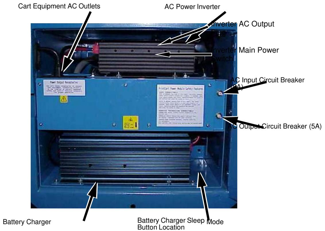
**Figure 9. Power Module (Inverter/Charger) Features and Safety Devices (230V PrintCart)**
