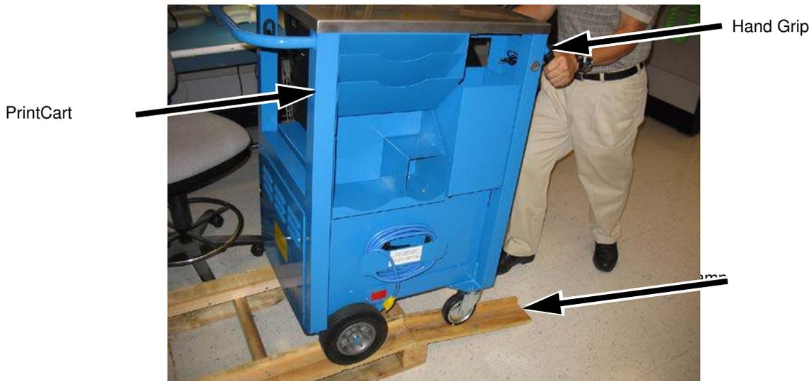
**Figure 3. Moving the PrintCart to the Work Surface**
