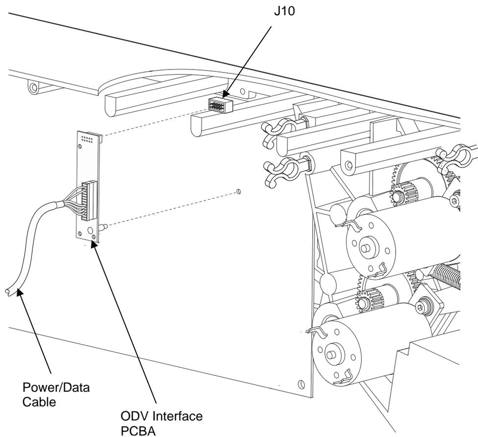
**Figure 17 Connecting the ODV PBCA and Controller (T8)**
