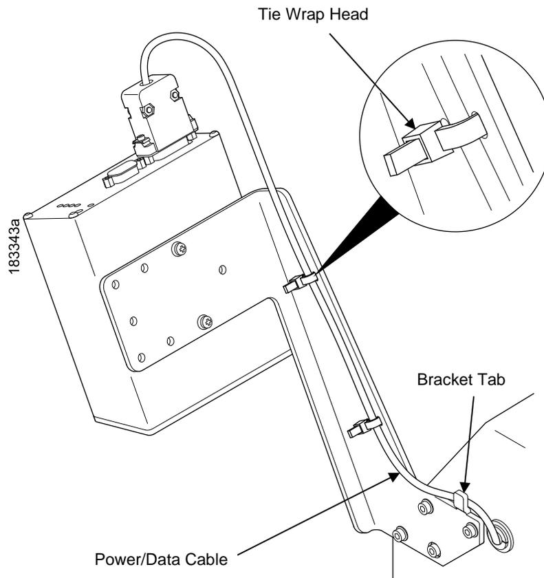
**Figure 22 Securing the Power/Data Cable (T8)**
