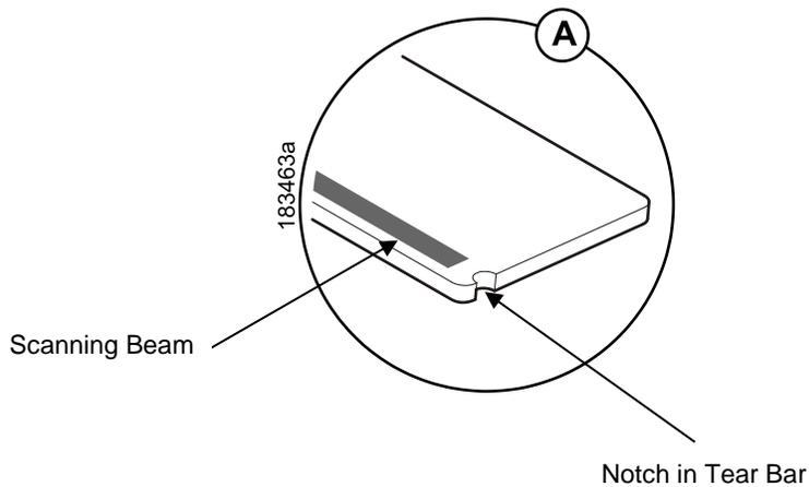
**Figure 25 Scanning Beam Location**
