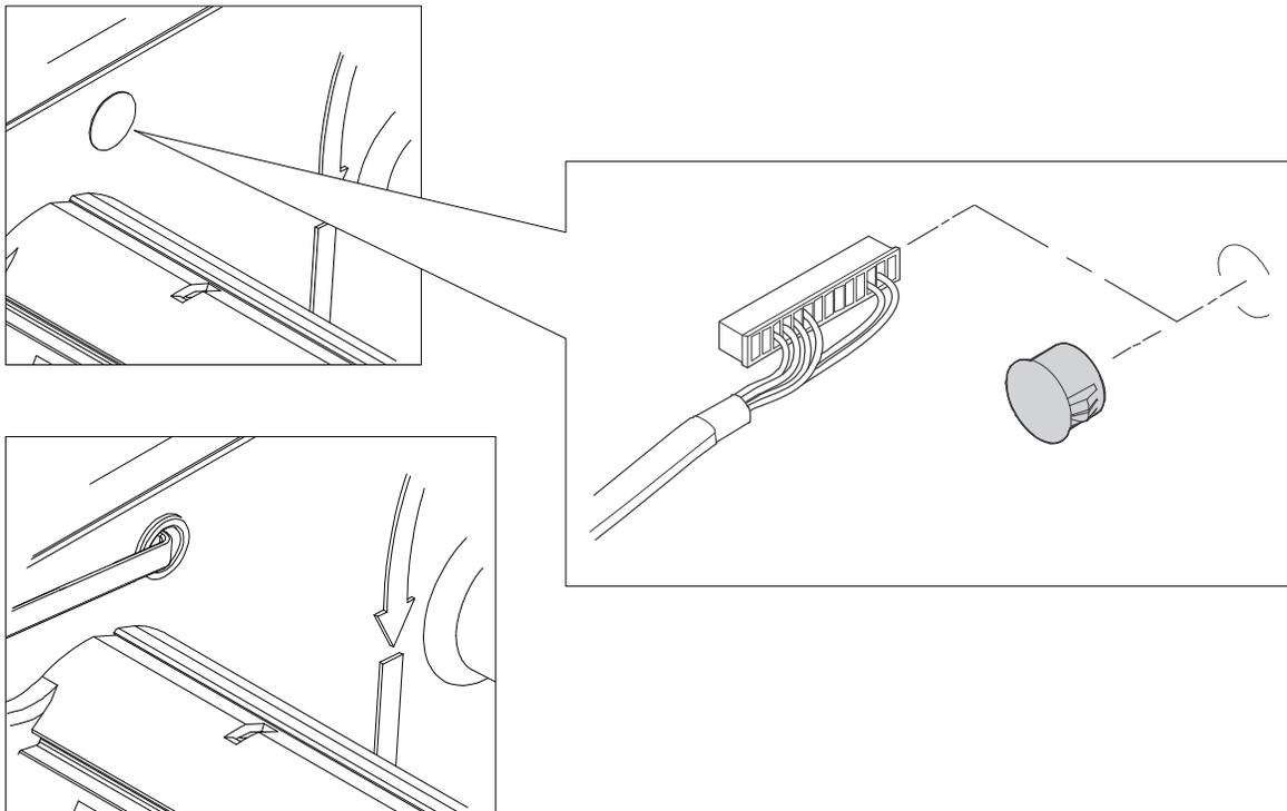
**Figure 3 Routing the Power/Data Cable (T6)**
