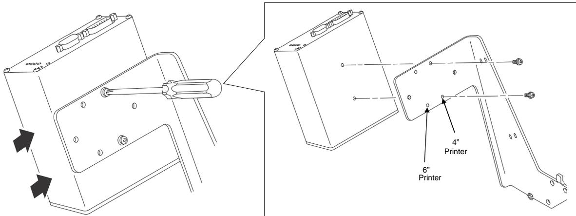
**Figure 6 Attach Validator to the Bracket (T6)**
