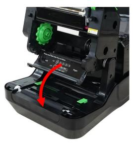
8. Push the right side of the ribbon rewind spindle to press the right spring-loaded spindle and then align the left side of the rewind spindle with the left spindle's hub ensuring that the ribs on the gear fits with the rewind spindle.
