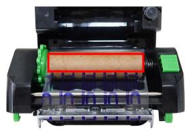
12. Rotate the gear in the indicated direction until the ribbon completely covers the printhead.
