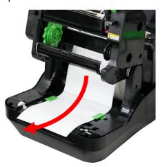
11. Adjust the media guides ensuring that the media guides fit with the width of the media.
