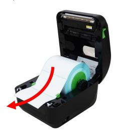
7. Adjust the media guides ensuring that the media guides fit with the width of the media.
