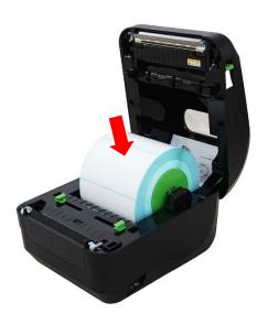
5. Rotate the media to make sure that the media is properly secured and rolls smoothly.
