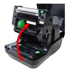
6. Secure the printhead mechanism in place.
