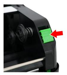
5. Open the printhead mechanism.
