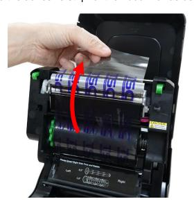
11. Carefully attach the adhesive strip on the rewind paper core.
