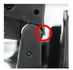
When using the black mark labels, adjust the location of the black mark sensor ensuring that the black mark sensor is aligned with the path of black marks.
