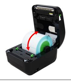
6. Feed the media in the indicated direction until it extends out of the front panel of the printer.
