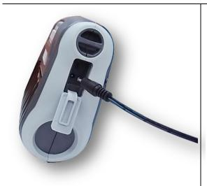
1. Open the interface cover and plug the power cord to the power jack.
