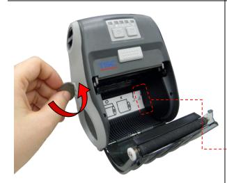
Use a coin to rotate the media holder adjustment knob, and the media holder should be placed at the correct place to fit the media roll.
