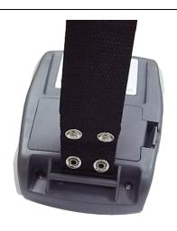
Refer to figure beside. Loop the belt clip through the slot below the battery.
