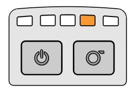
3. When the battery is charging, the color of battery status LED indicator is solid amber.
