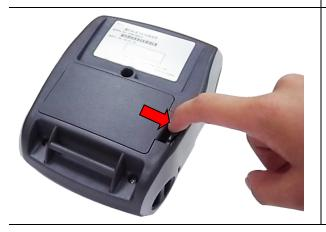
3. Pull the battery clasp to lock the battery.
