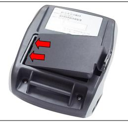
1. Insert the left side to install the battery at the rear of the printer.
