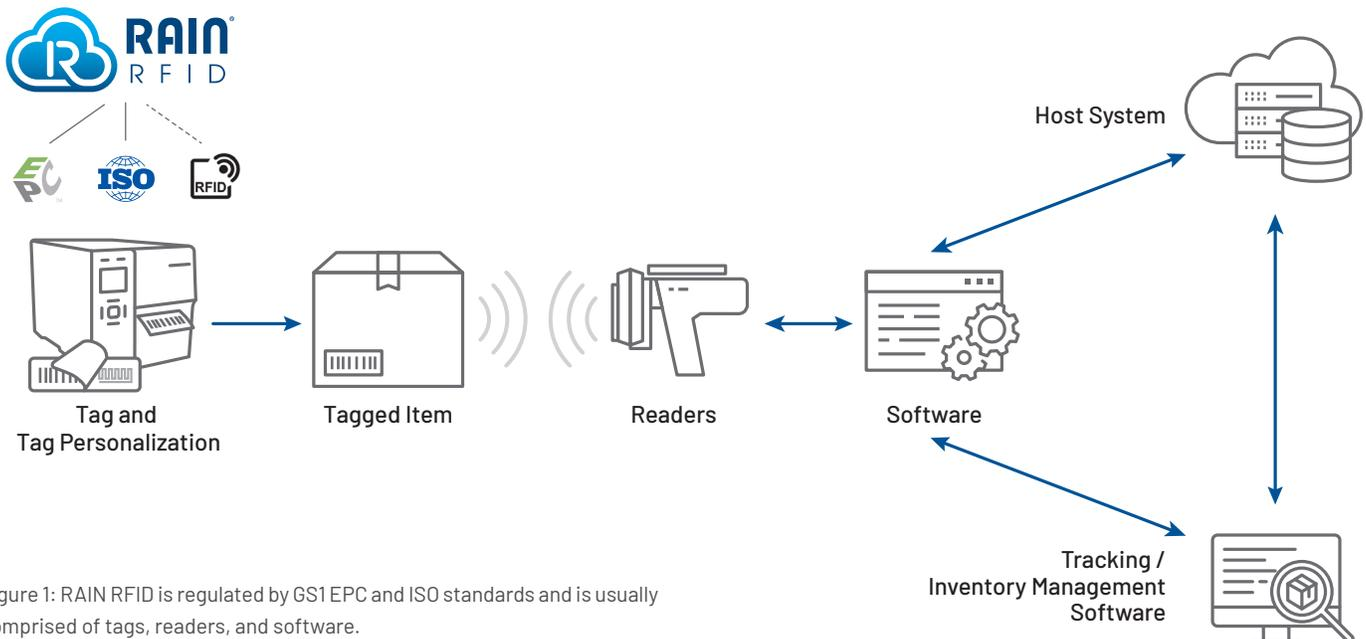
Figure 1: RAIN RFID is regulated by GS1 EPC and ISO standards and is usually comprised of tags, readers, and software.
